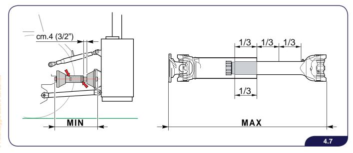
► Check that the length of overlap between the shaped pipes is not less than 2/3 of the stroke with the PTO shaft closed. Otherwise, cut the excess part of both the telescopic pipes (A) and the guards (B). Cut both sides the same length.
