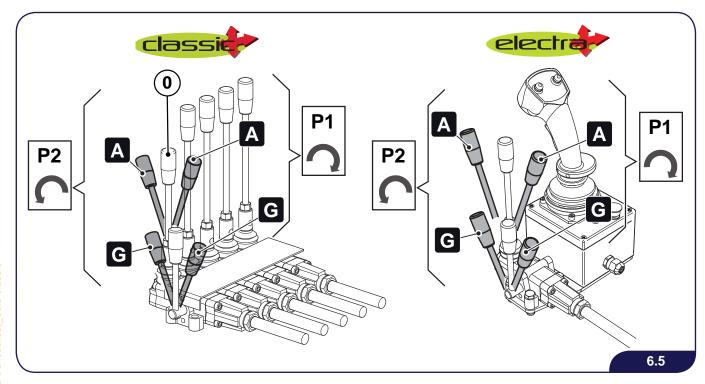
The lever **A** controls the rotation direction of the rotor. **Engage the lever G** in order to enable control for lever **A**.
